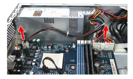
6. Remove the screw (D) that secures the power supply.
